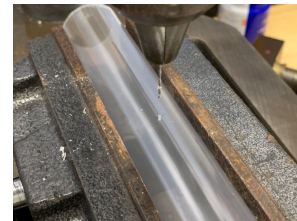
Fig. 40. Drilling holes at the sensor location
