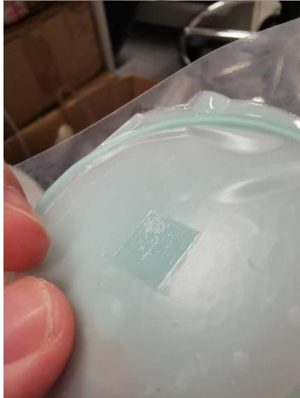
After creating the turnover mold, another kind of silica gel is used to make the actual part for application. The material is called Mold Star 15 Slow also produced by Smooth-On company. Simply mixing the part A and part B of the material and putting the turnover mold on to the material can create the parts we need as shown in the picture at the left.
