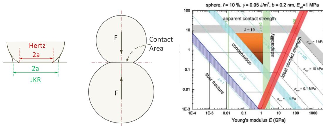
The theory can calculate the necessary force for producing a contact area with two different spherical solids of different radius.
