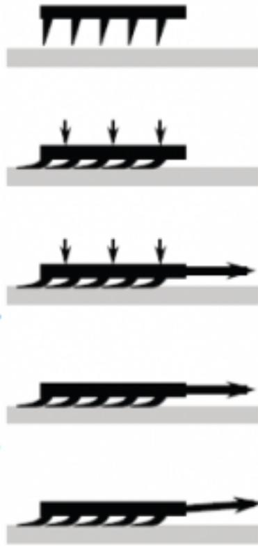
In this UROP project, the shape shown in the picture beside is used. Each spike looks like a right triangle. Technically, when providing a shear force and a normal force, the surface contact together will provide a relatively big van de Waals force. This force will drag the things to be gripped to the gripper.
