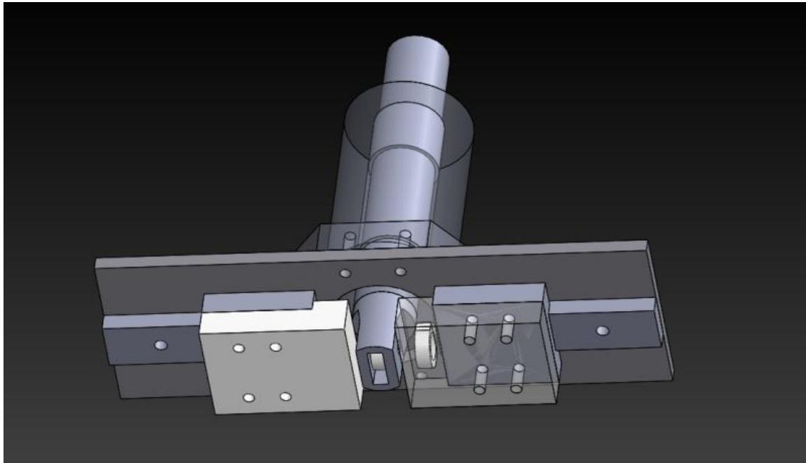
Despite the manufacture of the material, a mechanical gripper is also designed aimed to apply the material as a gripper. The mechanism is made of several parts, two separated mini rails is attached on a board and a rod pressed by the used is also attached on the same board. the two slider is hold with magnet. The magnets will always tend to
